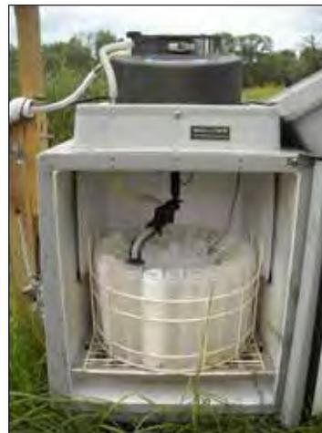
**Figure 6.** Automated, solar-powered samplers being inspected by Raj Patel, EPA Project Supervisor, during his August 2011 site visit. In- and out-flowing water was sampled and stored; each carousel rotated to accept sequential samples. Runoff from 13 storms (late 2011 through 2012) was analyzed water to assess removal of Total Phosphorus, Total Dissolved Phosphorus, Total Nitrogen, and Total Suspended Solids (TSS). Photo on left by Zedler; photo of auto-sampler by Prellwitz.
