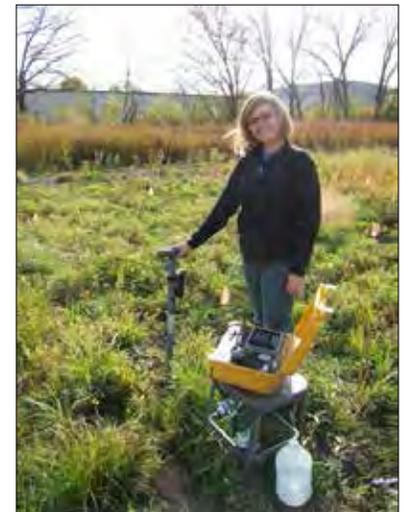
**Figure 4.** Prellwitz used a cohesive-strength meter to assess erosion resistance. Photo of Prellwitz by Z. Zopp.
