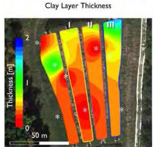
**Figure 2.** Clay was thickest in swale III, which held the most surface water. Mapped estimates based on only 9 soil borings. Imagery by J. F. Miller.
